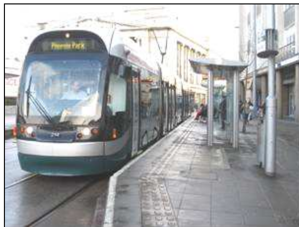
Plate 4.8: Minimal gap between platform and tram
