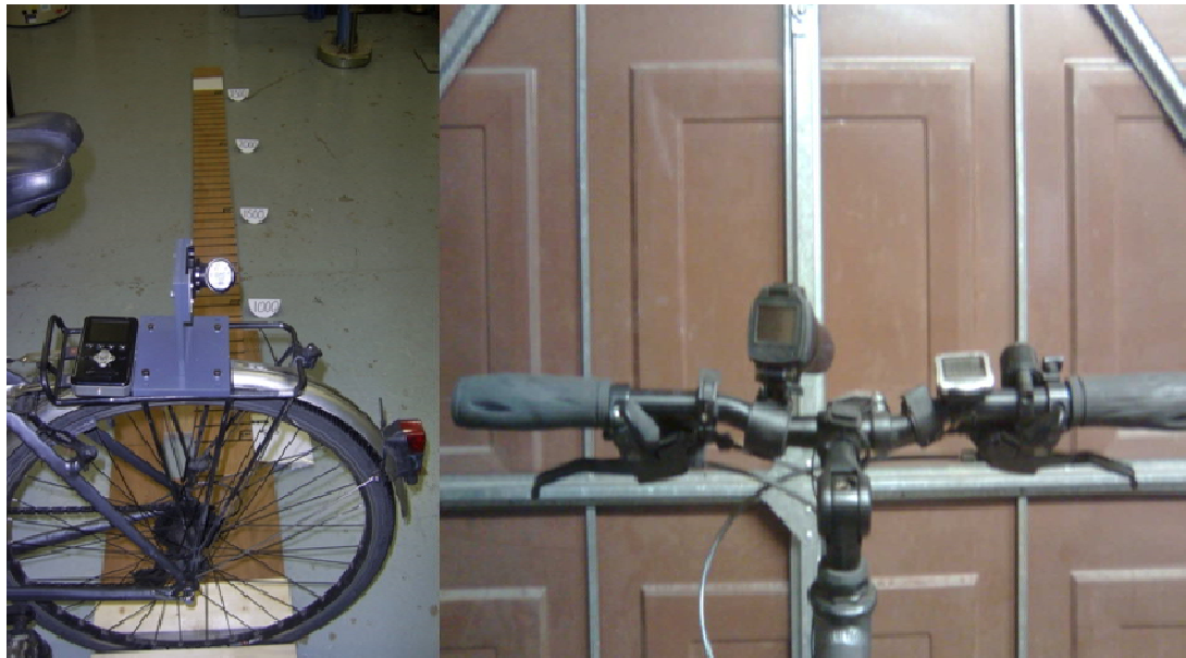
Photo 1 – Instrumented Bicycle, AT1 Camera/ Receiver, Mount, Cycle Stand and Graduated Board
