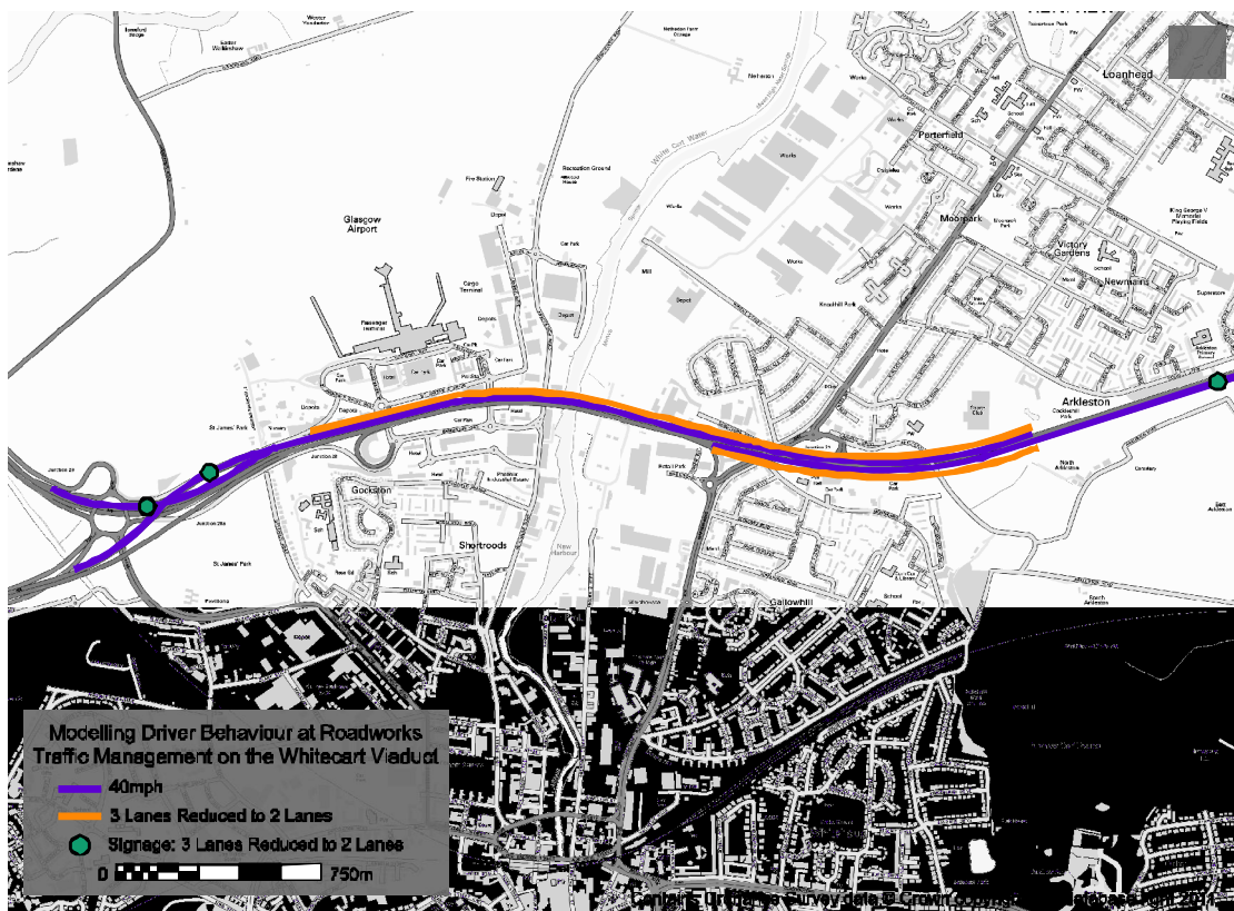
Figure 2.1 : Traffic Management on the Whitecart Viaduct
