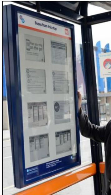
Figure 3 - Prototype E-paper Public Transport Information Display Unit
