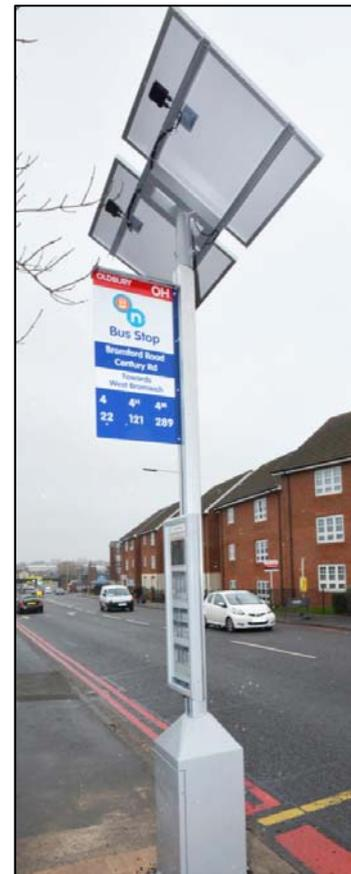
**Figure 6 – Prototype E-paper Public Transport Information Display Unit – Solar Power Trial**
