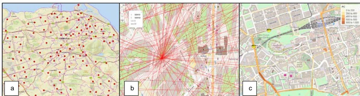
Figure 3. a) IZ with Population Weighted Centroids; b) Euclidean lines between O-D pairs; c) Route allocated flows from *splanr* and Cyclestreets.net
