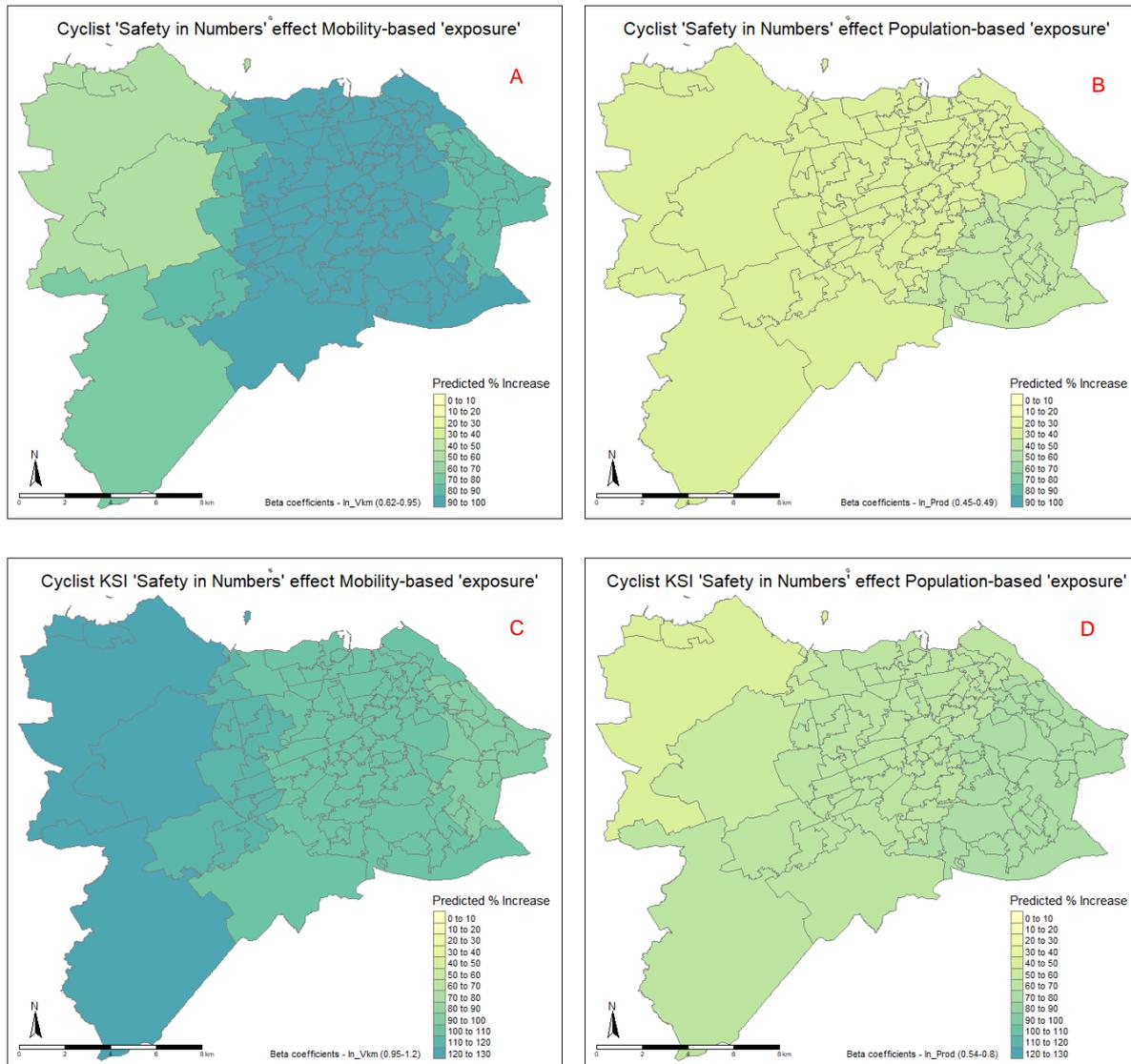
Figure 8. Percentage of expected collisions if cycling doubles with the modelled “Safety in Numbers” effect.
