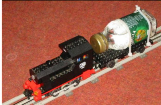
Figure 5: Lego locomotive with infra-red source
