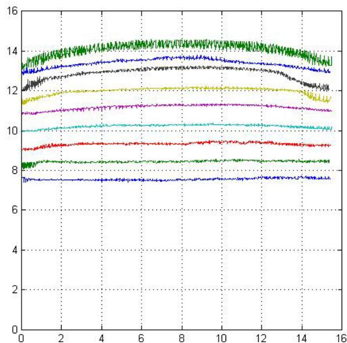
Figure 2 shows the effects of radial distortion. In contrast with the 'ground truth' where each of the above lines were ten centimetres apart, the lines in the data returned become more compressed the further they are from the centre of the lens. They also become increasingly curved, and suffer an increasing amount of noise in the data.
