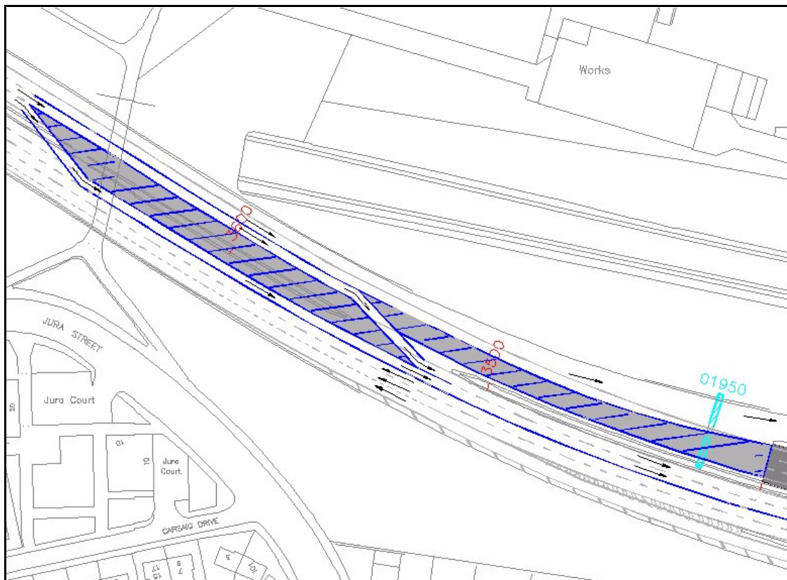
Figure 5: Example of Temporary Traffic Management Option: M8 Eastbound
